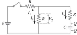
(a) At t = 0 the three currents canbe determined by analyzing asimpler, but equivalent, circuit.Identify this simpler circuit and use it to f
