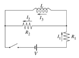
Determine the currents  $I_1, I_2, I_3$  in the resistors and in the self-inductor at the moment
