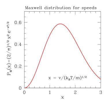
The probability tends to zero both for  $v \to 0$  and for  $v \to \infty$ . A characterisitic speed is  $\sqrt{k_B T/m}$  which is about 300 m/s for air. A problem in which you evaluate Gaussian integrals to determine several specific measures of the distribution is set in the homework.
