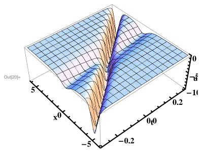
At negative times, the deeper soliton, which moves faster, approaches the shallower one. At t = 0 they combine to give  $u(x, 0) = -6 \operatorname{sech}^{2}(x)$ , (a single trough of depth 6) and, after the encounter, the deeper soliton has overtaken the shallower one and both resume their original shape and speed. However, as a result of the interaction, the shallower soliton experiences a delay and the deeper soliton is speeded up.
