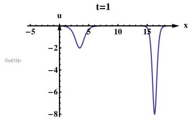
We see a trough of depth 8 and a trough of depth 2. To determine the speeds of these troughs we locate the minima of the function at two different times, t=2 and 3,
