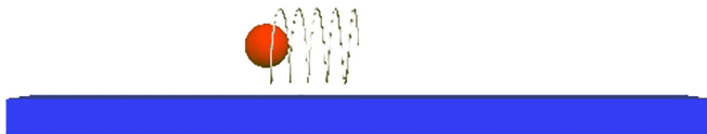
Fig. 5. A snapshot of a simulation of the Langevin equation, which models a particle in a highly viscous fluid coupled to a spring. This model is mathematically the same as that used to understand noise in optical traps. The graphics for this simulation were easily implemented using Visual Python 5 (enhanced online) [URL: http://dx.doi.org/10.1119/1.4869198.4 ].
