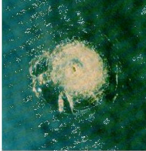
Windshield of the space shuttle damaged by a paint chip hurtling through space.
