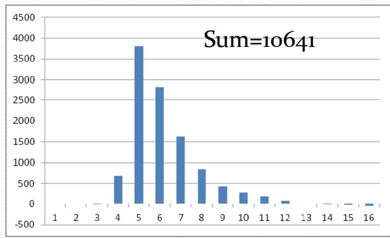
Some example energy detector measurements from a beam test last autumn. Each histogram represents a different absorber thickness used to slow down the protons.
