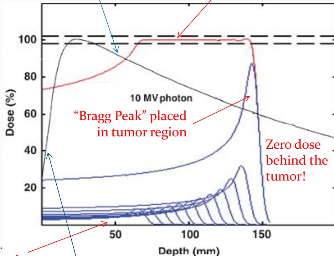
Energy deposition vs. depth for several beam energies.
