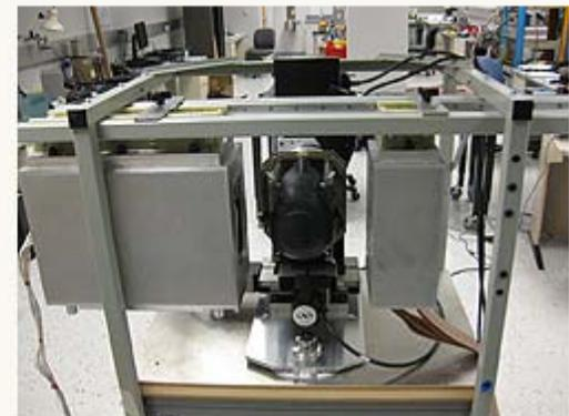
This prototype proton CT scanner was developed in the SCIPP laboratories by a team of physicists led by Hartmut Sadrozinski (below).
