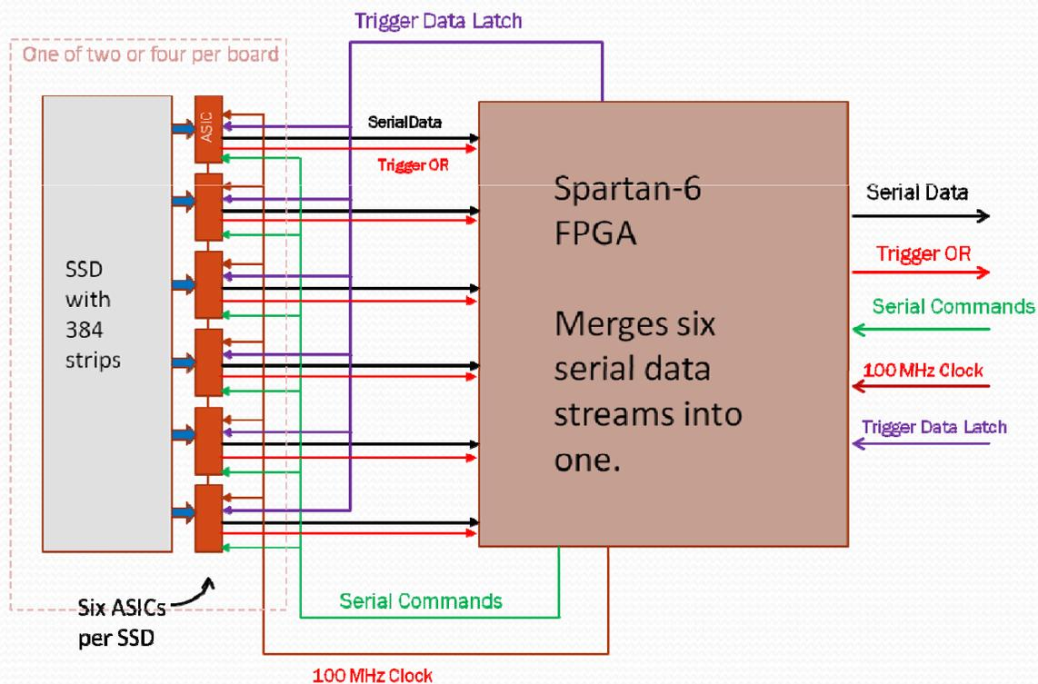
Six 64-channel amplifier chips per SSD.
