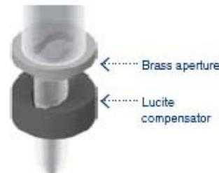
The brass aperture and the Lucite compensator are designed to squeeze the proton beam to the size and shape of the area being treated.
