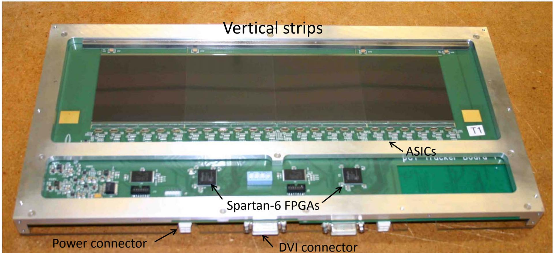
The T side has twice and many amplifier channels as the V side, and two FPGAs, each with a dedicated data line to the event builder.
