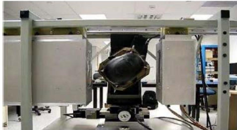
**Fig. 5.** Schematic sketch (left) and view (right) of the Phase I pCT scanner completed in 2010. The system consists of a front and rear module with a total of 4 silicon tracker planes and a crystal-calorimeter with an array of 18 CsI(Tl) crystals. The object (here a Rando head phantom) is rotating between the front- and rear-module on a rotational stage.
