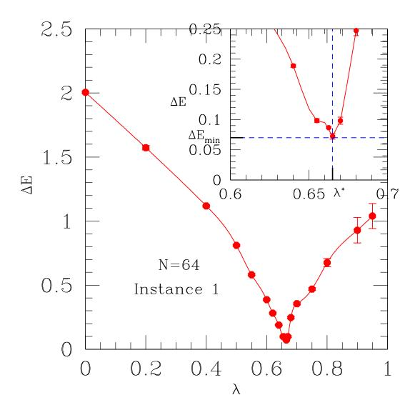
Results for the gap to the first excited state  $\Delta E$  as a function of the control parameter  $\lambda$  for one instance with N=64. The gap has is finite for  $\lambda=0$  (this is due to the driver Hamiltonian,  $\sum_i \sigma_i^x$ ). It is also finite for  $\lambda=1$  because we chose instances with this property (Unique Satisfying Assignment). There is a minimum of the gap at an intermediate value of  $\lambda$ , presumably close to a
