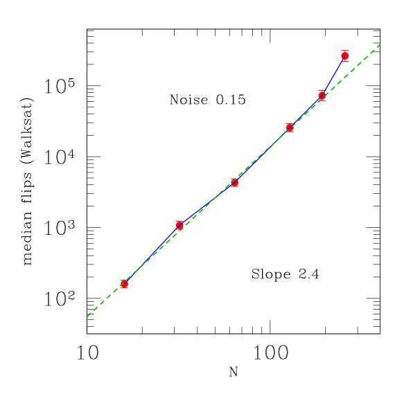
Adjusting the noise parameter, the crossover to exponential behavior is pushed to larger sizes  $N \gtrsim 200$ . (Remember: the QMC is so far only for  $N \leq 128$ ).
