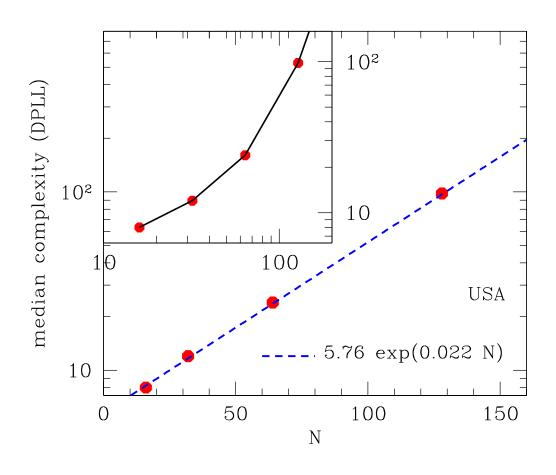
A commonly used classical algorithm for satisfiability problems is the Davis Putnum algorithm. This is guaranteed to correctly say whether or not there is a satisfying assignment. The figure shows the complexity for the instances used in the QMC simulations. It is clearly exponential for the range of sizes studied.
