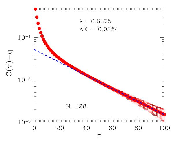
Results for the time dependent correlation function against  $\tau$  for one instance of the Exact Cover problem with N=128 near the location of the minimium gap. Note that the vertical axis is logarithmic. Fitting to the straight line region gives a slope (equal to the gap  $\Delta E$ ) equal to 0.0354.
