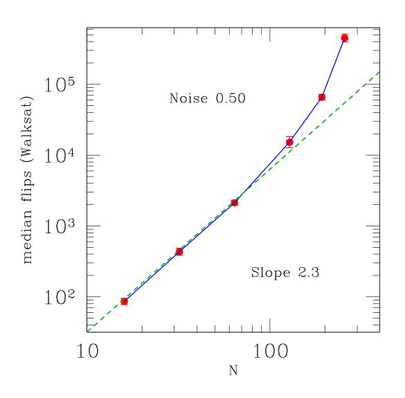
A classical algorithm which is more analgous to QAA is WALKSAT, a local heuristic search algorithm. Like simulated annealing, it includes "uphill" moves in a stochastic way. Using the default value of the "noise parameter" the complexity for the QAA instances with USA crosses over from power-law to (presumably) exponential for  $N \gtrsim 100$ . (But note the QMC is so far only for N < 128).
