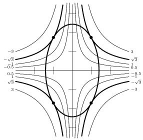
The ellipse is the level curve of g(x,y). The other curves are all various level curves of f(x,y), and the extreme values occur when these level curves share a tangent with the level curve of g(x,y). (These tangent level curves are darker than the other level curves of f.)
