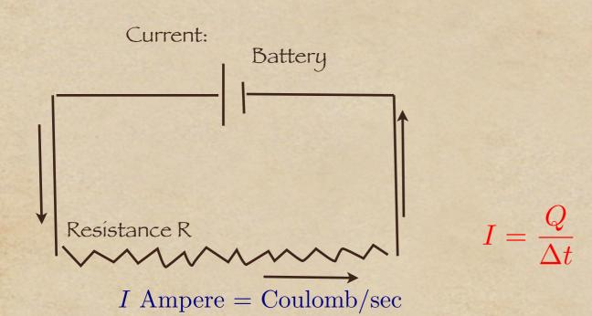
Useful Analogy: Charge "Q" is the total quantity of water in a tank. Current "I" is the amount of water flowing through a pipe per second Unlike charge, the current has a direction. We may speak of Q as a scalar and I as a vector.
