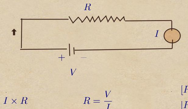
True for most metallic wires R= resistance of the wire
